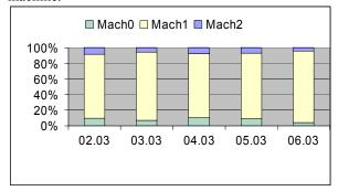
Figure 1 shows the percentage of packets received per honeypot. The unequal repartition is mainly due to the different OS behaviors. Mach1, the NT server, is a lot more responsive than mach0 and mach2. We are also surprised to observe how constant the packets repartition remains over the months.
